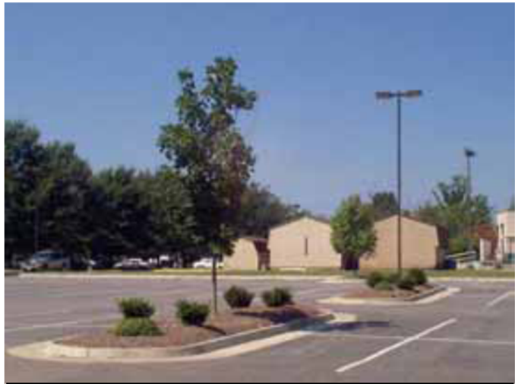
Trees and lights should be separated from each other, especially in parking lots, to avoid causing shadows.
